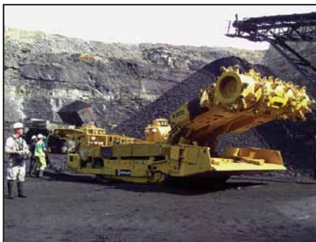
**In extremely hot and dusty conditions, the operator, above at left, uses a Hetronic RRC to easily control a mining machine.**
